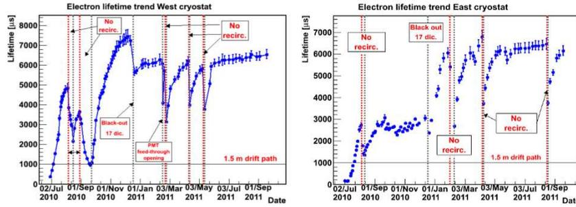
Fig. 2. Free electron lifetime evolution with time in 2010-2011 run, for both cryostats.
