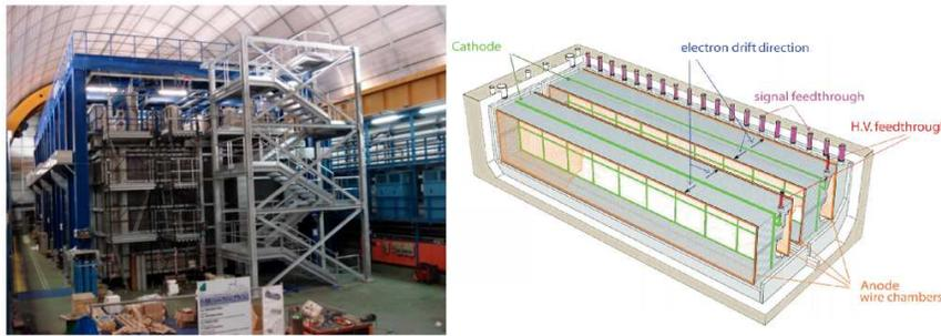
Fig. 1. The ICARUS T600 detector in Hall B at the LNGS underground laboratory (left) and a simple sketch of the inner TPCs structure (right).
