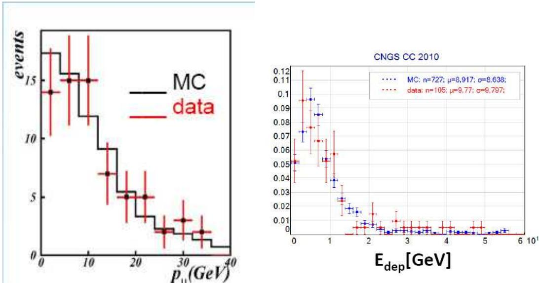
**Figure 3:** Left: momentum spectrum of muons from  $\nu_{\mu}$  CC interaction reconstructed by multiple scattering, compared with MonteCarlo. Right: distribution of the total deposited energy in  $\nu_{\mu}$  CC interaction events, compared with MonteCarlo.
