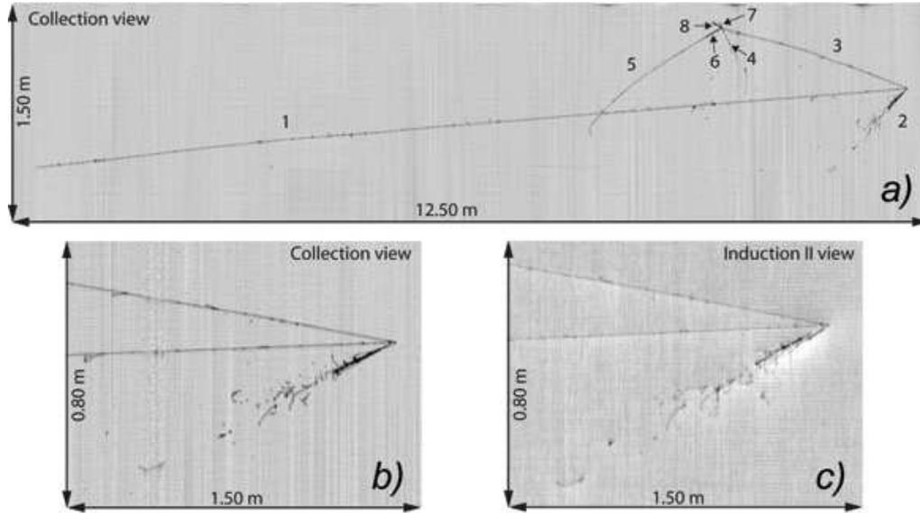
Figure 2: An example of  $\nu_\mu$  CC interaction from the CNGS beam in Collection view *a)*; a close-up view of the primary vertex for the Collection *b)* and Induction-2 *c)* projections allow solving completely the event topology.
