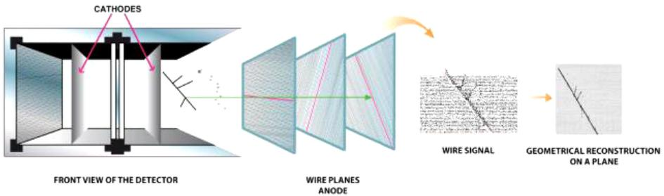
Fig.1. Illustration of the ICARUS T600 working principle: a charged particle ionization path in LAr and its geometrical reconstruction on a plane.
