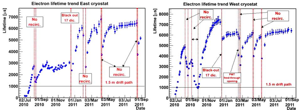
Fig. 2. Free electron lifetime monitoring in East (left) and West (right) cryostats as a function of the elapsed time.
